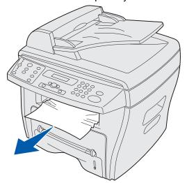
3 If there is any resistance when you pull the paper, or the paper is not seen in the front output tray, open the rear cover.
